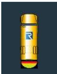
ROSS indicators are Green for no object detected, Amber for object intrusion and Red for Stop. Varying Beep Sound intensity will occur based on object position. Solid tone occurs when the Red Indicator is enacted and will not shut off until reverse trigger power is cycled on and off. Object size and velocity are determining factors in distance at which the indicators activate.
