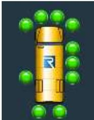
Once the SDS zones are active the green indicators on the SDS Display Unit will be ON. The areas of coverage will vary based upon installation of the sensor.
