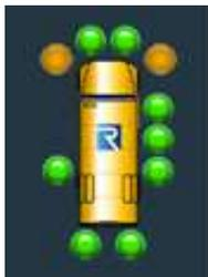
In the event of lost sensor communication 2 amber icons will begin to flash and the display will sound an audible alarm. This alarm will continue until the fault is cleared. This typically occurs when a sensor is damaged or harness is severed or shorted.
