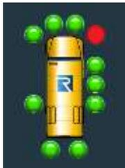
The audio alarm will beep for one second EVERY instance of object movement within any of the SDS zones and the corresponding green indicator will change to red. The red indicator will flash for a minimum of five seconds after the intrusion has cleared, or until activation signal is removed.
