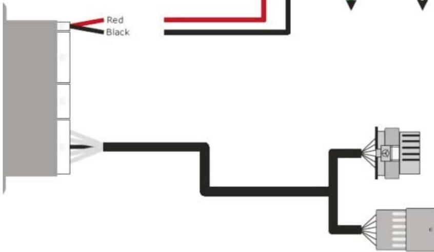
Connector on the accelerator pedal
